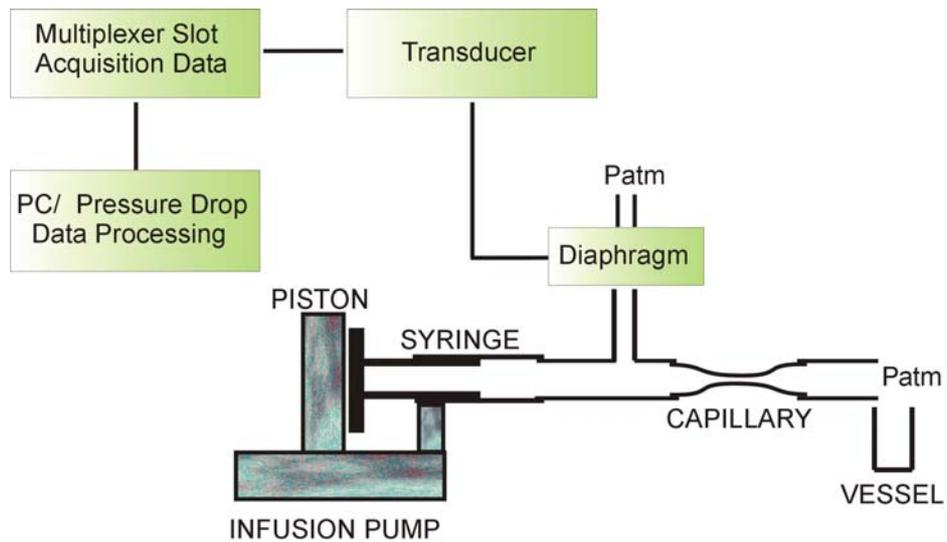
Figure 5. Acquisition system for measuring pressure drop data.
