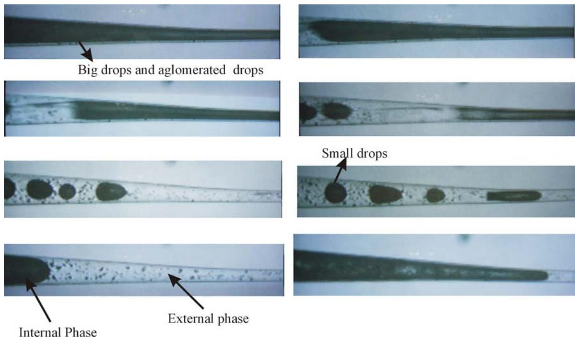
Figure 10 . Visualization of emulsion 2L flowing through the constriction.
