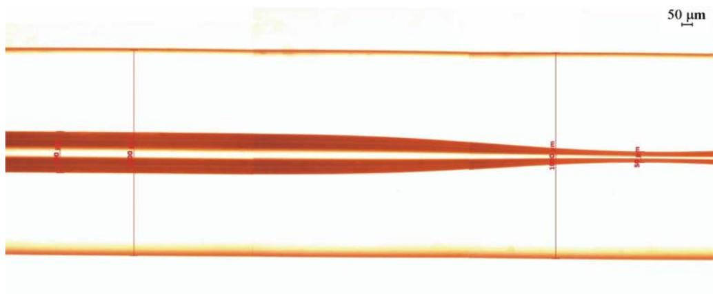
Figure 6. Glass capillary used in experiments. ( $200\ \mu\text{m}$  in diameter and  $50\ \mu\text{m}$  in constriction).
